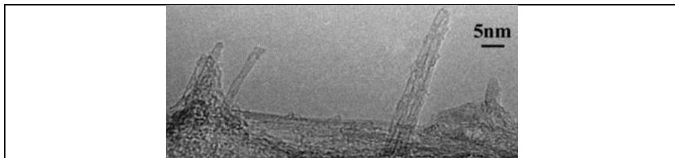
Fig. 3. HRTEM image of an SWNT filled with Fe nanoparticles introduced from \text{Fe}(\text{NO}_3)_2 solution at room temperature with subsequent annealing at 300^\circ\text{C}
